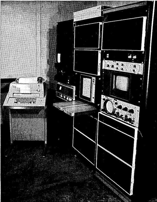
Fig. 4. PDP8/I computer system.
